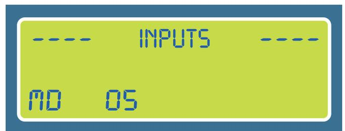
They are voltage-free inputs and they can only be detected when the specific input is connected to the input common through the controller.
