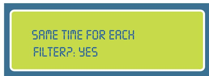
If we press  the controller will ask for a single CLEANING and PAUSE time, while if we press , the controller will ask for the value for each filter and pause.
