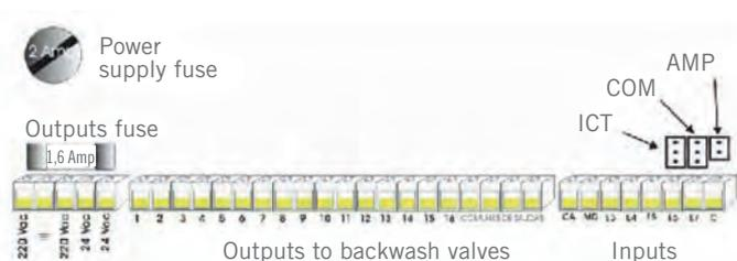
We connect here all electrical wires to external devices to be controlled or from external devices providing information to the controller.
