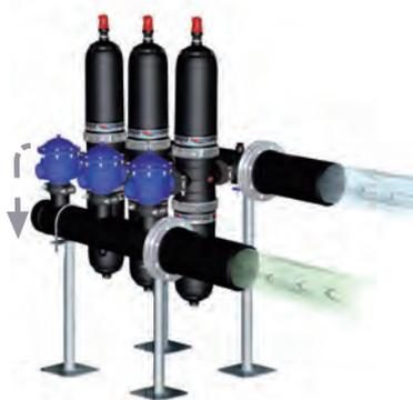
Our range has different filtration degree color-coded discs depending on the total suspended solids of raw water to be filtered and our automatic filtration stations are designed to match flow requirements of the installation. The cartridge spine has an internal piston spring for compressing or releasing the discs during the filtration and backwash cycles.
